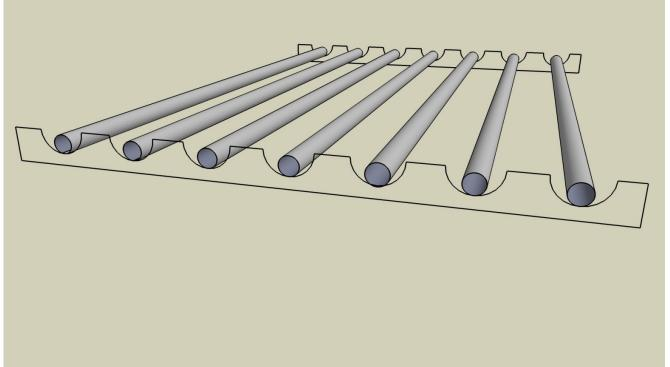
Fit the smoke dowel brackets to the inside walls at the desired heights using 25mm screws at 100mm spacing.
