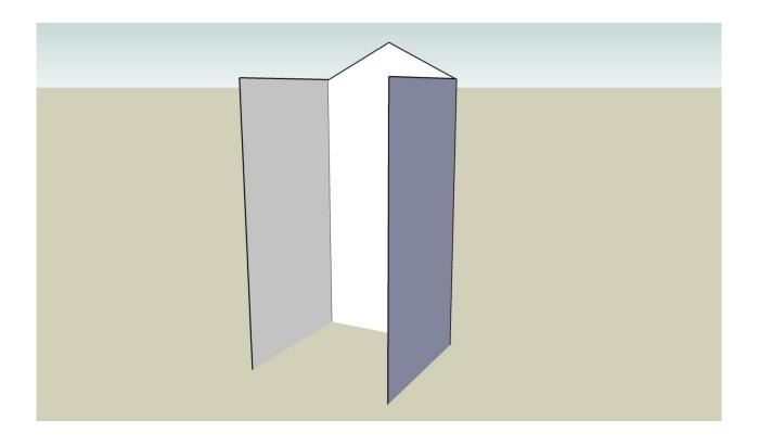
Take the two front door pillars Drill holes through the wall edge 8mm in at 200mm spacing with the 3mm drill bit, down the full length of one side and do the same with the other piece.
