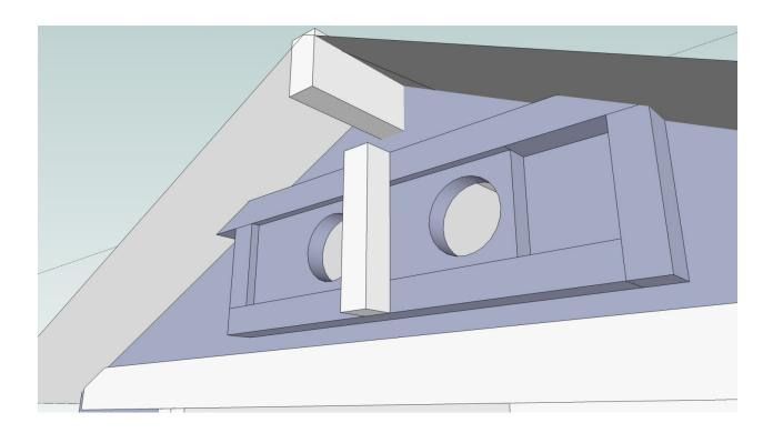
Your project is nearly complete, cut a 60mm hole in the centre of one of the side for your Smoke Cannon 350mm from the base using the hole saw.
